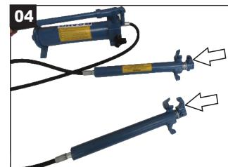
Open valve Right to Left, using hands only expand the rods.
